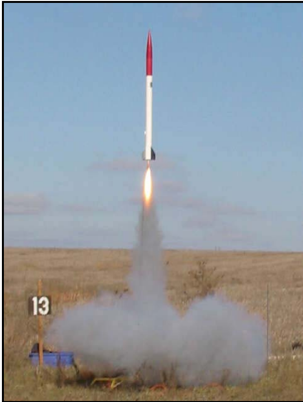
Liftoff on a G64. Though the parachute hung up, the Arcas was undamaged and flew again.
