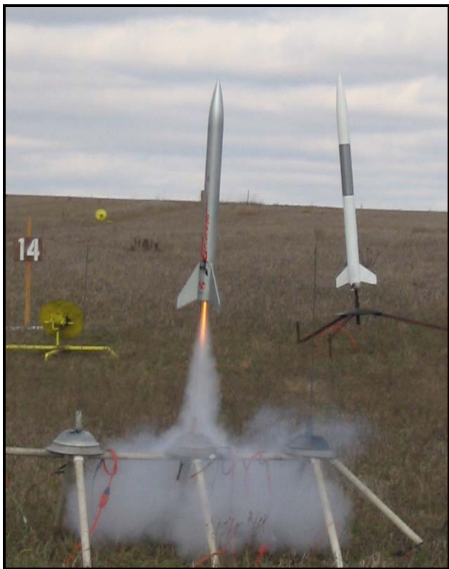
Liftoff on a D12-3. Steven's Executioner was flown several more times on E9's and an F39.
