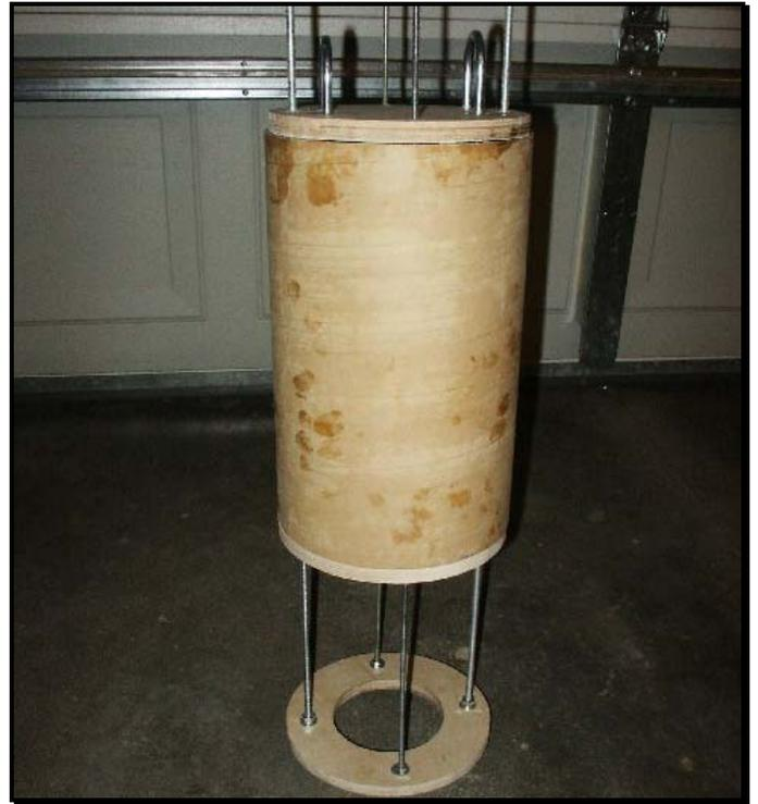
This is the shoulder assembly for the fin canister section of *Blazing Glory*. (Rothman)
