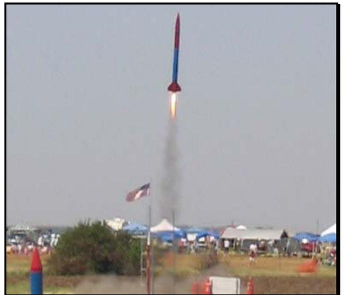
*Aquarius* flew Saturday on a Hypertek M1000... motor of choice of many non-LEUP, Level 3 flyers at LDRS! Sometime after powered flight, the epoxy of the Slimline retainer weakened and the whole motor fell out ruining a successful flight. Ouch! (Burney)
