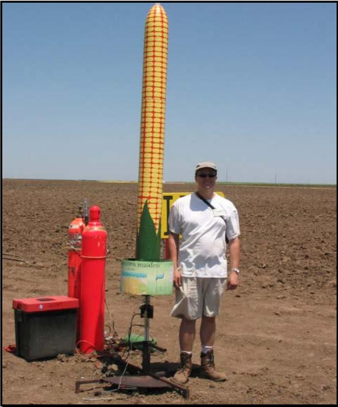
Kevin poses with *Lusty*. Unlike *Lusty's* flight at LDRS XXI, the timer was to be triggered by its gravity switch and not by pull pin. Motor for this flight would again be a Hypertek M1000. (Burney)
