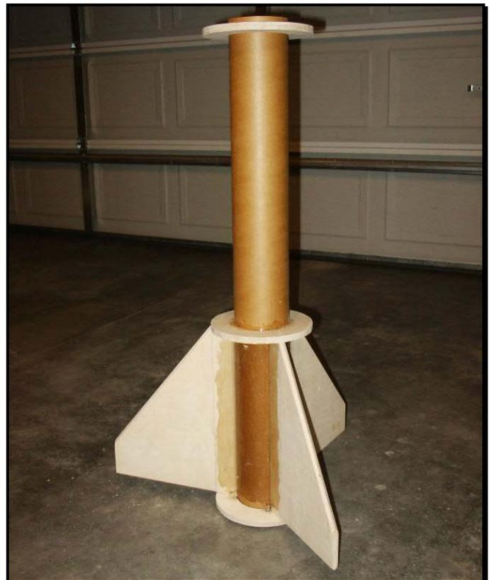
The fin and motor mount assembly. The plywood fins are thick... either 3/8" or 1/2"! (Rothman)
