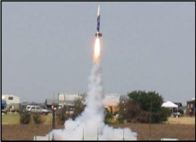
Liftoff on an AeroTech K700, which happens to be the largest motor I've flown to date. This was also the first time I used both an altimeter and timer for deploying two separate ejection charges; my first completely electric flight! (Burney)
