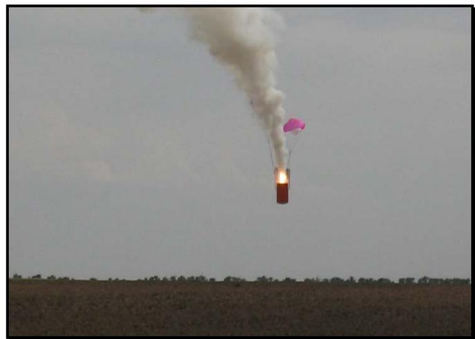
Flight sequence of *Our Stinkin' Rocket*. At liftoff, the twin parachutes came out prematurely causing the rocket to not even break 100 feet even with two AeroTech M1419's. Landing was hard, but *Our Stinkin' Rocket* is repairable and will fly again!
