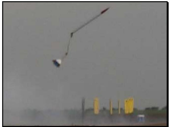
Flight sequence of *Maxie D*. Unlike Larry's *Mini Max*, the flashpan ignition only lit about 140 of the 316 motors resulting in a grossly underpowered flight. The timer separated the main sections just before it hit the ground. Though the rocket was pretty banged up, *Maxie D* will probably be rebuilt.
