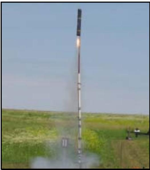
Liftoff on a Pro38 G69. Due in part to it being underpowered, the rocket only got up about 50 feet.
