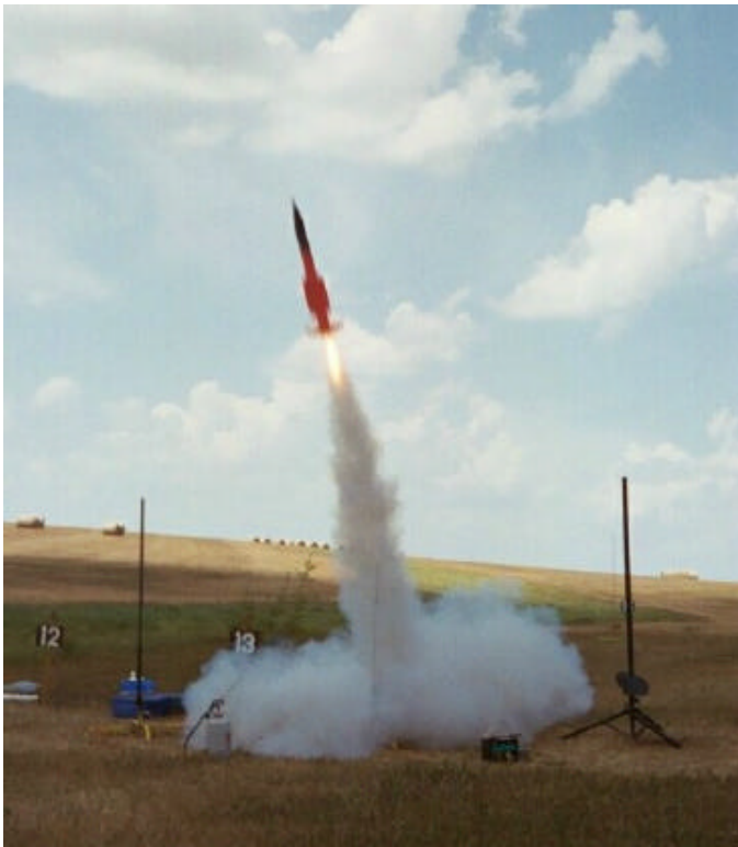
Liftoff! After the Archer cleared the pad, it took a cruise missile trajectory to the west due to an uneven ignition sequence of the motor cluster.
