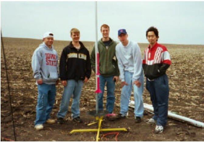
Some students from Iowa State who are part of an aviation program at that college, built and designed a minimum diameter rocket powered by an F39 reload. What looks like an upper stage is an unpowered "dart" which drag separates from the booster after motor burnout. This has got to be the smallest rocket that I have seen that uses a launch rail! The first flight resulted in a recorded altitude of 800-900 feet (altitude was recorded using a Perfect Flight M9K). Another flight took place later.
