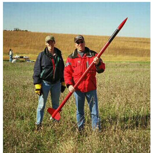
**Jason Burton and Greg Rothman with Greg's Level 2 attempt. Powered by a J350, Greg's rocket had a magnetic apogee censor for main deployment and two tracking transmitters (one belonging to the club and one belonging to him).**
