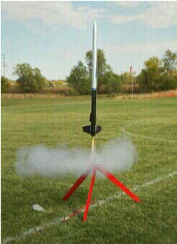
**A slow, but yet vertical takeoff. Some models that have marginal flights on motors like the D12-3, may want to steer clear of the low thrusting E9... my Shadow suffered a bad zipper after the 4 second delay ended up being way too much.**
