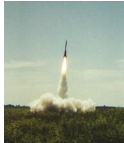
Takeoff! The first few seconds of flight were awesome, but the PML Quantum tubing wasn't strong enough for the stress on the side pods which ripped off and then the rest of the vehicle came apart.
